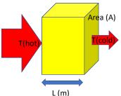
Q = K x A x [ T(hot) – T (cold)] / L Q/A = K x dT /L Q/A = dT/( L/K) = dT / R
